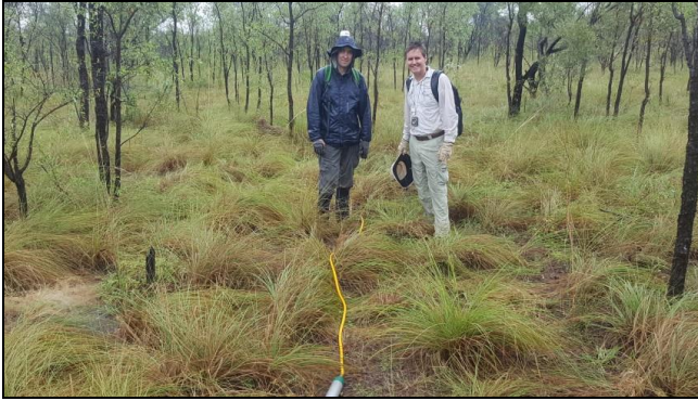
POZ Chairman Jim Richards and geophysicist Mathew Cooper conducting the GPR Survey at Blina in 2017. GPR tool is the yellow 'snake' to front. DGPS carried by operator.
