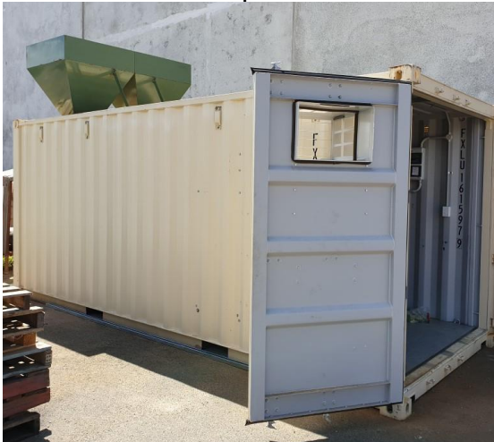
Concentrate feed hoppers on roof of Sortex unit. Feed in via Sanko conveyor
