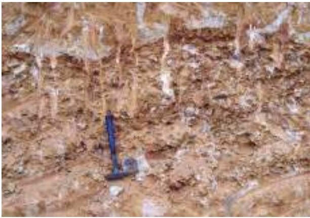
Figure 25. Example of clast-supported gravels overlying bedrock comprising highly weathered fine- to medium-grained feldspathic quartz sandstone (photo by GMI Rockett)
