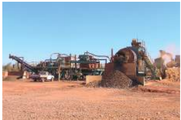
Figure 60. Blina Diamonds' 50-tph dense-media separation production plant (photo by D Jones)
