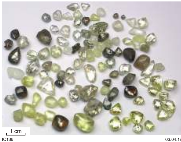
Figure 35. A 152.43 ct parcel of +13 to +23 DTC (Diamond Trading Company round-hole sieve series) stones recovered from the E12 Alluvials trial mining (photo by GMI Rockett)
