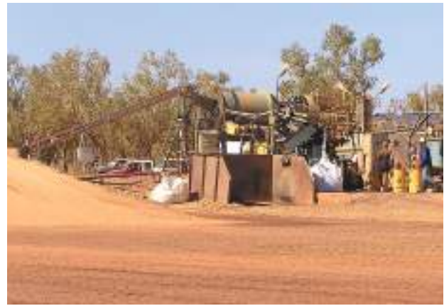
Figure 59. Blina Diamonds' 10-tph dense-media separation exploration plant (photo by D Jones)
