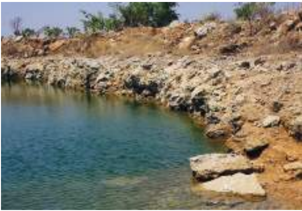
Figure 21. Photo of a pit in E4S exposing the calcrete cap on the top of the pipe (photo by G Boxer)
