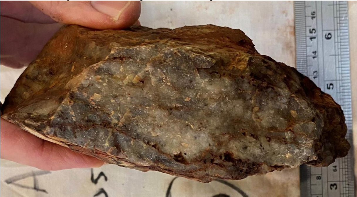
Rock Float Sample ER005 shows quartz boudinaged vein of the so-called 'kidney reef' style which has been widely reported at Edjudina. This sample assayed 2.11 ppm Au
