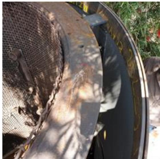
Note the rotating inner 14mm screen is a sleeve within the 3.15mm outer screen. This configuration allows simultaneous sizing and dewatering within the one unit and is attached to and powered by the trommel assembly. The oversize is transited out of the unit via an extension sleeve (not shown in photo).
