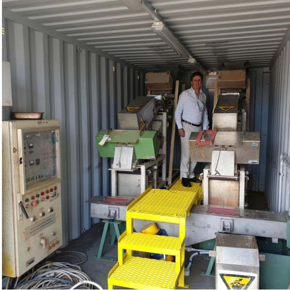
Dual array diamond Sortex recovery system built by POZ using Ellendale Sortex machines. Control panel on LHS
