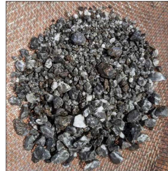
IQRC 001 (137-138m) Galena and sphalerite mineralisation assayed 8.9% Zn & 12.7% Pb
