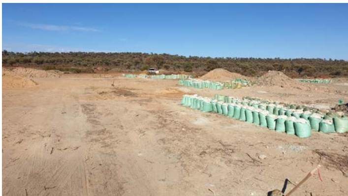
Neta Lodes Phase 3 RC drilling samples, calico one metre 'splits' sample bags sit on top of the green cyclone bags
