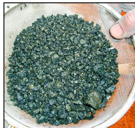
Manchegeo Phase 1 drilling: RC Drill Chips from MRC 040 (74-75m) showing sulphide mineralisation within gabbro-norite host
