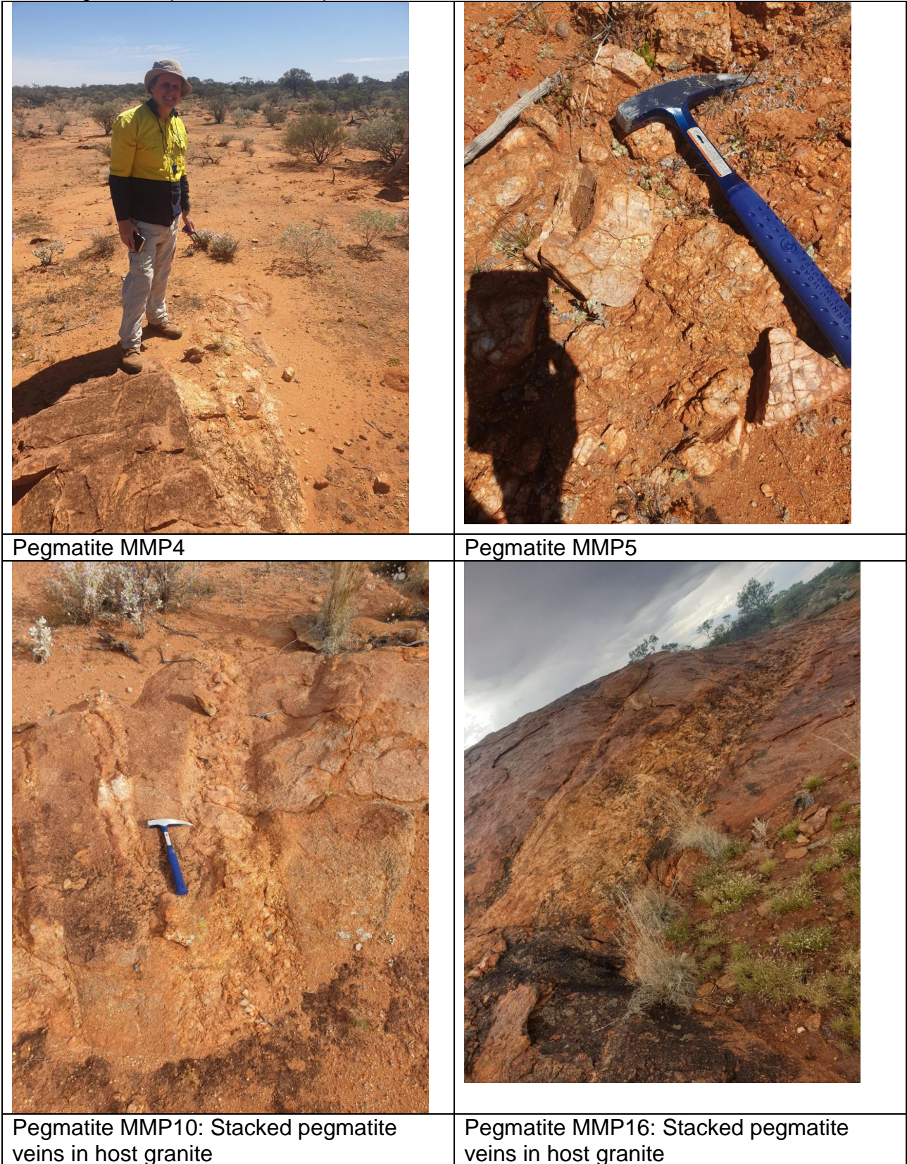
Figure 3: Mount Magnet East Lithium Project - Pegmatites Coarse grained quartz and feldspar with muscovite +/- biotite
