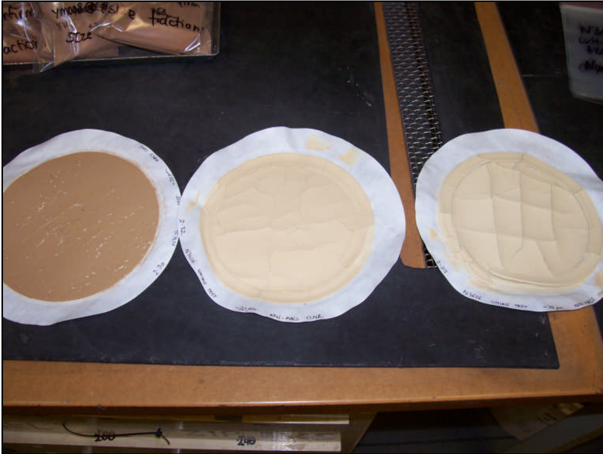
Photo 1: Products from fines WHIMS testing. Iron rich residue on left. Samples to right are the non-magnetic fractions (phosphate rich).
