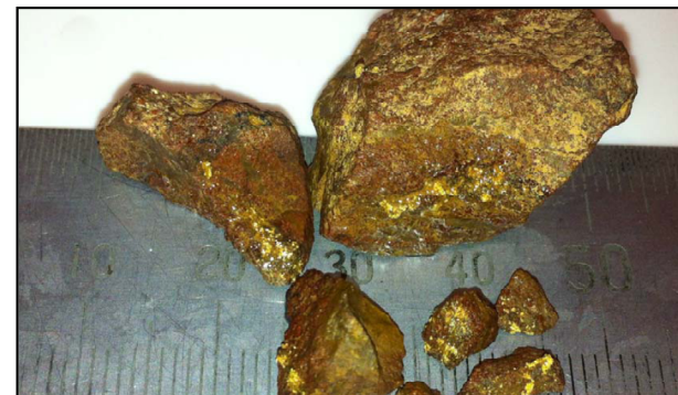
POZ aircore hole PAC 142, 6- 7metres - native gold on aircore drill chips. Assayed at 776g/t Au
