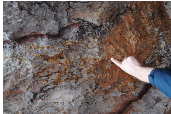
Rock chip sample GER 01 taken from roof of the Mount Lucky workings. Quartz veining in sheared sericite-limonite-argillic alteration.
