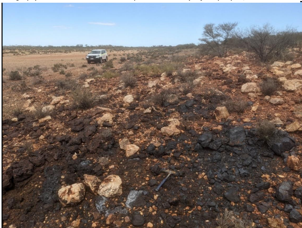
Figure 2: Malecite prospect - outcropping gossan (black-dark brown) in relation to the Iroquois dolomite breccia (white – cream) – looking south-west. Peak results of 7.3% Pb, 0.5% Cu, 4.8g/t Ag, 0.4% Zn and 25% Mn were returned from rock chip sample assays
