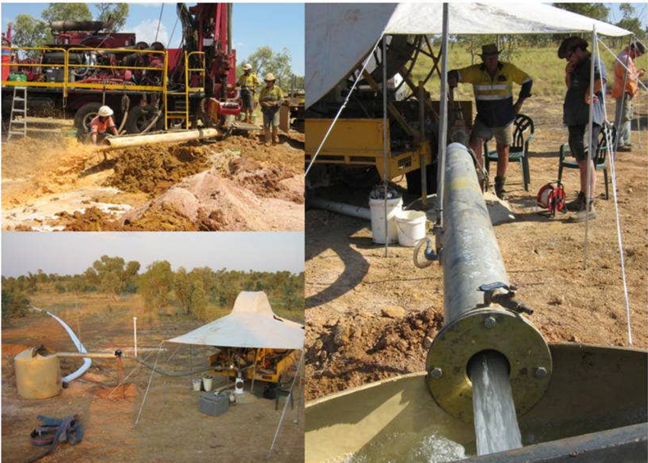
Photo 1: Drilling and Pump Testing WB02.
